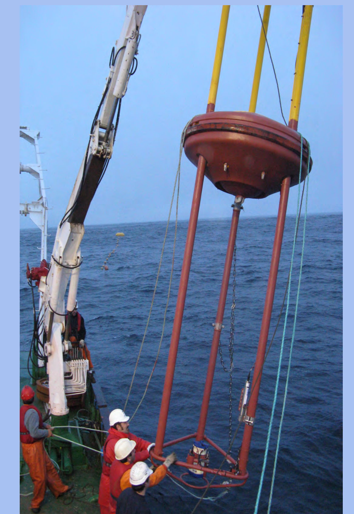
Deployment of the AGL Buoy after ordinary maintenance
